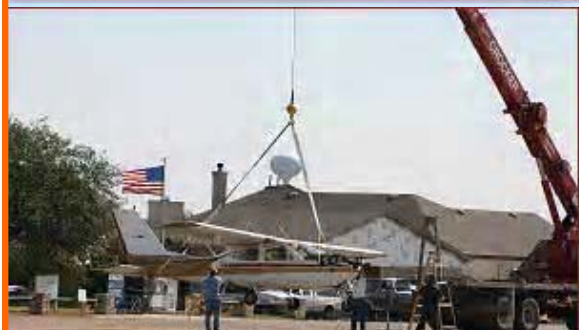
Crain lifting airplane into the air to enable gear to be extended
