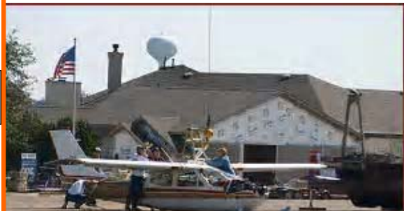
Cessna RG after gear up landing awaiting lift to put the gear down
